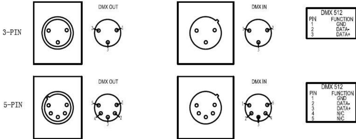
Connection between the controller and a projector and between one projector and another must be made with a 2 core-screened cable, with each core having at least a 0.5mm diameter. Connection to and from the projector is via cannon 3 pin (which are included with the projector) XLR plugs and sockets. The XLR's are connected as shown in the figure above.
