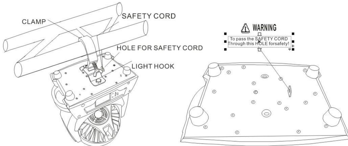
Use 1pcs clamp and safety cord(need to purchase).Use clamp fix with light hook which in the packing box with light, then use screw install to the bottom of lamp. Hang the fixture on the structure and fasten the screws attached to each clamp. Make sure the light is installed reliable, and confirm the light which you fixed is strong enough for hanging the light. Base on safety reason, please according to the above picture using safety wire cross the light to make it strong enough again.
